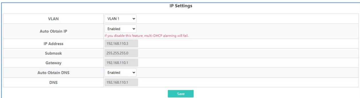
When VLAN Settings is set to on, select the management VLAN from the configured VLANs (you can choose **VLAN Settings > VLAN Members** to add a VLAN).
