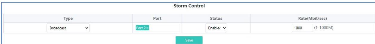
**Display part:** The storm control types and rates configured for device ports are displayed (when storm control is enabled, the storm control rates are displayed).
